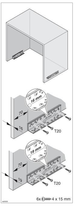
■ Screw the brackets onto the right and left inside walls of the housing unit so that they are flush with the bottom edge of the wall unit.
